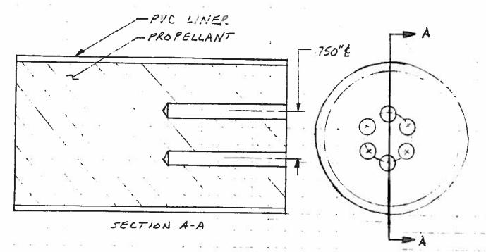
DRILL SIX EQUALLY SPACED .250"DIA HOLES CENTERED ON A .750" CIRCLE
