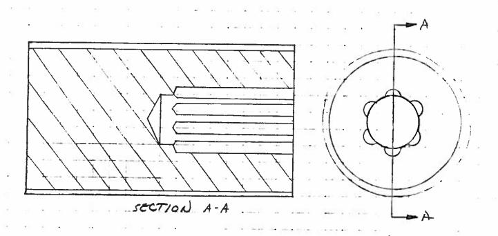
NEXT, DRILL A .750 DIA, HOLE CONCENTRIC WITH THE CENTERLINE CIRCLE OF THE .250" DIA HOLES. DRILL THE .750" DIA HOLE ABOUT .250 DEEPER THAN THE .750"DIA. HOLES.
