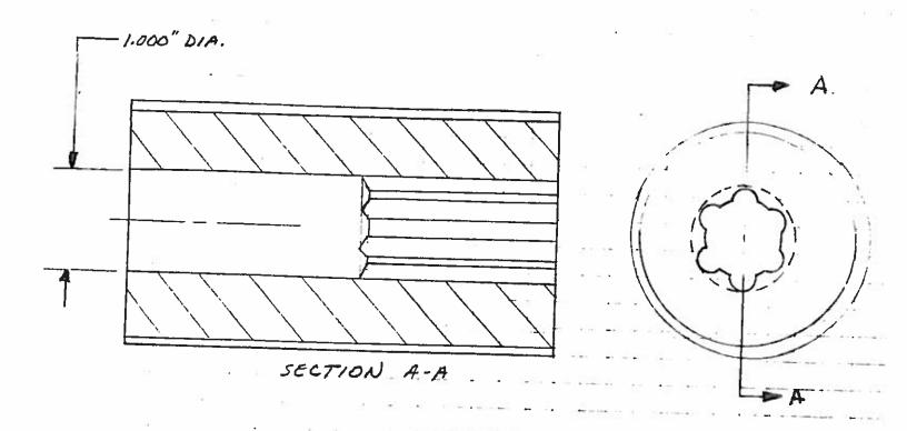
LAST, DRILL THE 1.000 DIA. GRAIN BORE HOLE TO THE BOTTOM EXTENT OF THE 250 DIA HOLES.
