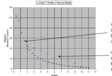
Clark-Y airfoil produces lift over limited range of "negative" angle of attack, so the twist angle must carefully follow effective air stream direction
