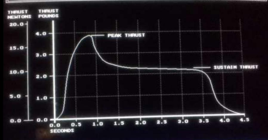
THE PEAK THRUST OF THE MOTOR IS THE HIGHEST POINT ON THE THRUST-TIME CURVE. THE PEAK OF THIS MOTOR IS ABOUT 3.9 Lbs. (17.4 Ht.)
