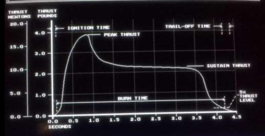
THRUST RISES TO 5% OF ITS PEAK VALUE, TO WHERE IT DECLINES TO 5% OF ITS PEAK VALUE, TO WHERE IT DECLINES TO 5% OF ITS PEAK VALUE. THIS HETHOD PREVENTS BURN TIMES FROM BEING DISTORTED BY SLOW IGNITION OR EXCESSIVE THRUST TRAIL-OFF TIME. THE BURN TIME OF THIS HOTOR IS ABOUT 4.1 SEC.
