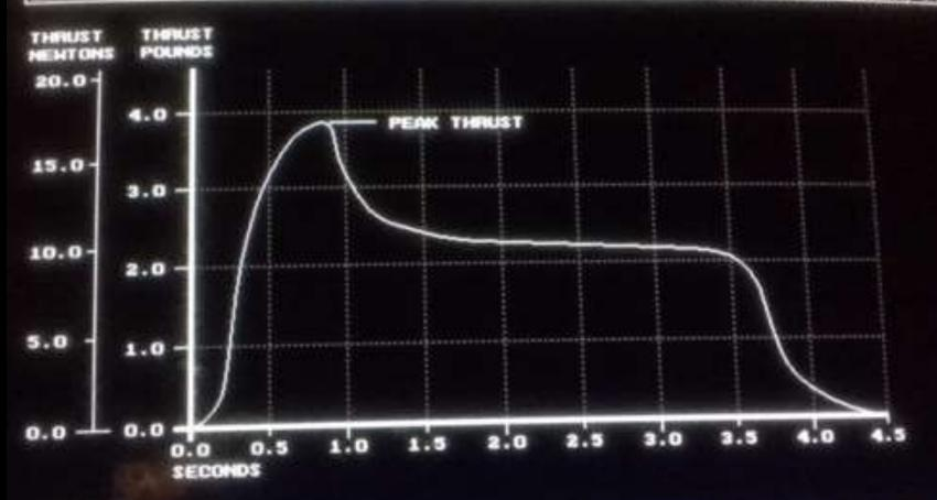
THE PEAK THRUST OF THE MOTOR IS THE HIGHEST POINT ON THE THRUST-TIME CURVE. THE PEAK OF THIS MOTOR IS ABOUT 3.9 Lbs. (17.4 Nt.)
