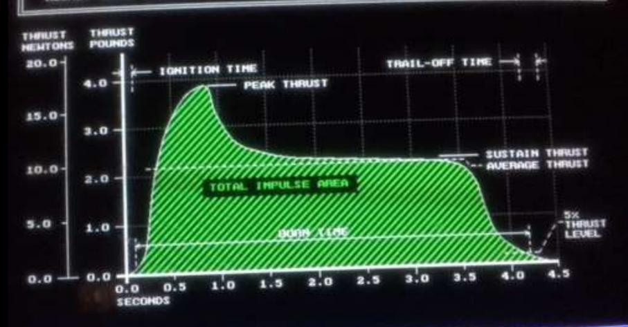
THE AVERAGE THRUST OF A MOTOR IS ITS TOTAL IMPULSE DIVIDED BY ITS BURN TIME. THE AVERAGE THRUST IS AN INDICATION OF HOW QUICKLY A MOTOR WILL ACCELERATE A ROCKET. (CAUTION: THE PEAK AND SUSTAIN THRUST SHOULD ALSO BE CONSIDERED WHEN DETERMINING THE SUITABILITY OF A PARTICULAR MOTOR.) THE AVERAGE THRUST OF THIS MOTOR IS ABOUT 2.1 Lb., OR 9.3 Nt.
