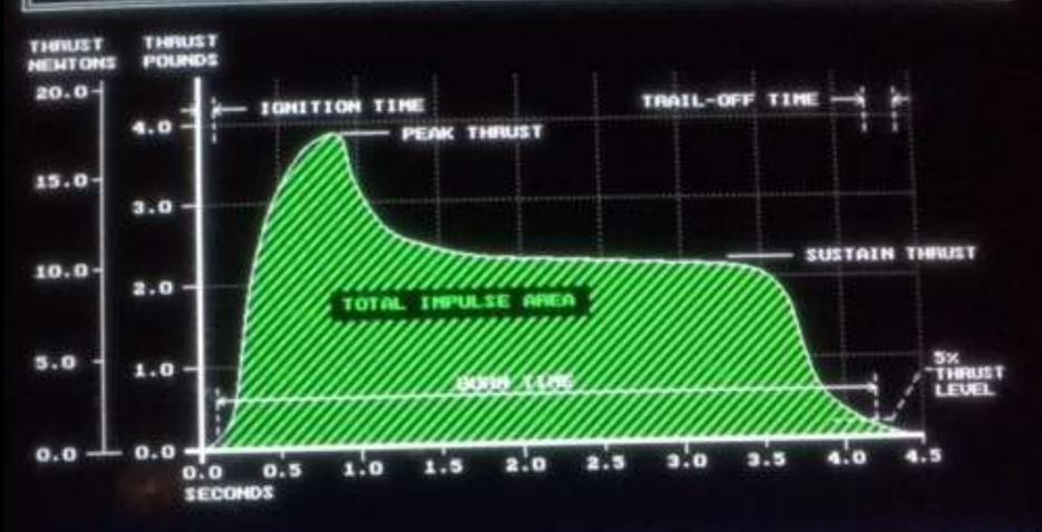
THE TOTAL IMPULSE OF A MOTOR IS THE TOTAL AREA UNDER THE THRUST-TIME CURVE. SINCE THE AXES ARE IN UNITS OF FORCE AND TIME, TOTAL IMPULSE IS HEASURED IN UNITS OF LB-SEC (ENGLISH), OR NEWTON-SEC (METRIC). TOTAL IMPULSE IS A MEASURE OF THE TOTAL ENERGY CONTAINED IN THE HOTOR. THE TOTAL IMPULSE OF THIS HOTOR IS ABOUT 9.8 LB-SEC, OR 44 NT-SEC.
