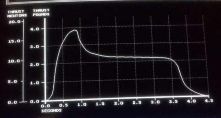
DIFFERENT MOTORS HAVE DIFFERENT THRUST-TIME CURVE SHAPES. THIS IS THE TYPICAL SHAPE OF OF A PARTIALLY CORED BLACK PONDER MOTOR. OTHER THRUST-TIME CURVE SHAPES WILL BE PRESENTED WITH THEIR RESPECTIVE MOTOR ANIMATIONS.
