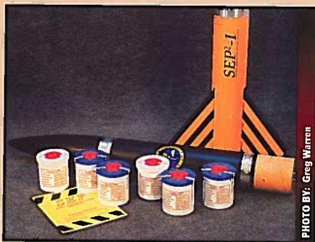
SEP 1 with typical manifest for one flight. Each canister contains one experiment.
